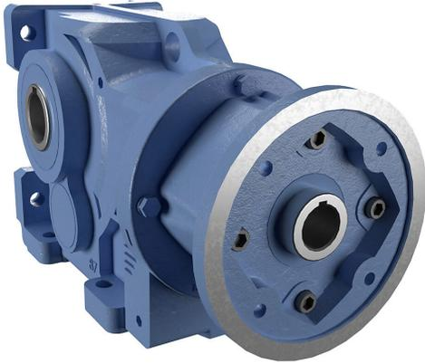
IronHorse heavy-duty helical bevel gearbox, 20:1 ratio, 254/6TC-Face input, hollow, 2.375in diameter output shaft, nominal 20hp at 1.29 SF, 17650 lb-in mechanical output torque, Type-87 frame, cast iron housing, vertical or horizontal mount.
