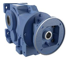
IronHorse heavy-duty helical bevel gearbox, 20:1 ratio, 213/5TC-Face input, hollow, 2.375in diameter output shaft, nominal 10hp at 2.59 SF, 17650 lb-in mechanical output torque, Type-87 frame, cast iron housing, vertical or horizontal mount.
