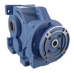
IronHorse heavy-duty helical bevel gearbox, 120:1 ratio, 143TC-Face input, hollow, 2in diameter output shaft, nominal 1hp at 3.42 SF, 12480 lb-in mechanical output torque, Type-77 frame, cast iron housing, vertical or horizontal mount.
