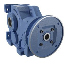
IronHorse heavy-duty helical bevel gearbox, 80:1 ratio, 182TC-Face input, hollow, 2in diameter output shaft, nominal 3hp at 1.79 SF, 13710 lb-in mechanical output torque, Type-77 frame, cast iron housing, vertical or horizontal mount.
