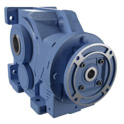
IronHorse heavy-duty helical bevel gearbox, 80:1 ratio, 143/5TC-Face input, hollow, 2in diameter output shaft, nominal 2hp at 2.69 SF, 13710 lb-in mechanical output torque, Type-77 frame, cast iron housing, vertical or horizontal mount.
