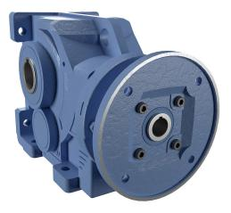
IronHorse heavy-duty helical bevel gearbox, 60:1 ratio, 182/4TC-Face input, hollow, 2in diameter output shaft, nominal 3hp at 2.39 SF, 13325 lb-in mechanical output torque, Type-77 frame, cast iron housing, vertical or horizontal mount.
