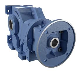
IronHorse heavy-duty helical bevel gearbox, 40:1 ratio, 213TC-Face input, hollow, 2in diameter output shaft, nominal 7.5hp at 1.23 SF, 11955 lb-in mechanical output torque, Type-77 frame, cast iron housing, vertical or horizontal mount.
