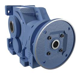
IronHorse heavy-duty helical bevel gearbox, 40:1 ratio, 182/4TC-Face input, hollow, 2in diameter output shaft, nominal 5hp at 1.84 SF, 11955 lb-in mechanical output torque, Type-77 frame, cast iron housing, vertical or horizontal mount.
