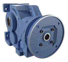
IronHorse heavy-duty helical bevel gearbox, 20:1 ratio, 182/4TC-Face input, hollow, 2in diameter output shaft, nominal 5hp at 2.96 SF, 9765 lb-in mechanical output torque, Type-77 frame, cast iron housing, vertical or horizontal mount.
