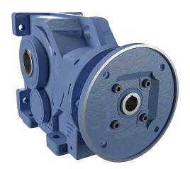
IronHorse heavy-duty helical bevel gearbox, 10:1 ratio, 182/4TC-Face input, hollow, 2in diameter output shaft, nominal 5hp at 4.8 SF, 7800 lb-in mechanical output torque, Type-77 frame, cast iron housing, vertical or horizontal mount.
