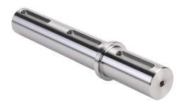
IronHorse gearbox single output shaft, 1.5in. For use with HBR-67 series gearboxes. (3) keys, (1) end plate, (1) lock washer and (1) bolt included.
