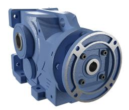
IronHorse heavy-duty helical bevel gearbox, 120:1 ratio, 143TC-Face input, hollow, 1.5in diameter output shaft, nominal 1hp at 1.88 SF, 7260 lb-in mechanical output torque, Type-67 frame, cast iron housing, vertical or horizontal mount.
