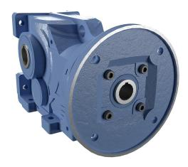
IronHorse heavy-duty helical bevel gearbox, 40:1 ratio, 182TC-Face input, hollow, 1.5in diameter output shaft, nominal 3hp at 1.54 SF, 5730 lb-in mechanical output torque, Type-67 frame, cast iron housing, vertical or horizontal mount.
