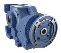
IronHorse heavy-duty helical bevel gearbox, 40:1 ratio, 143/5TC-Face input, hollow, 1.5in diameter output shaft, nominal 2hp at 2.31 SF, 5730 lb-in mechanical output torque, Type-67 frame, cast iron housing, vertical or horizontal mount.
