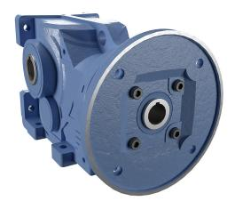
IronHorse heavy-duty helical bevel gearbox, 20:1 ratio, 182/4TC-Face input, hollow, 1.5in diameter output shaft, nominal 5hp at 1.25 SF, 4530 lb-in mechanical output torque, Type-67 frame, cast iron housing, vertical or horizontal mount.
