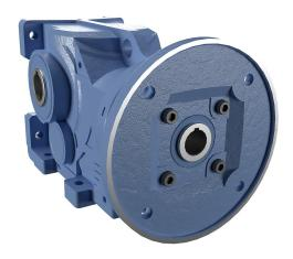
IronHorse heavy-duty helical bevel gearbox, 10:1 ratio, 182/4TC-Face input, hollow, 1.5in diameter output shaft, nominal 5hp at 2.41 SF, 3800 lb-in mechanical output torque, Type-67 frame, cast iron housing, vertical or horizontal mount.
