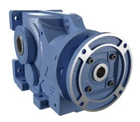
IronHorse heavy-duty helical bevel gearbox, 10:1 ratio, 143/5TC-Face input, hollow, 1.5in diameter output shaft, nominal 2hp at 6.03 SF, 3800 lb-in mechanical output torque, Type-67 frame, cast iron housing, vertical or horizontal mount.
