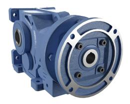
IronHorse heavy-duty helical bevel gearbox, 60:1 ratio, 143TC-Face input, hollow, 1.375in diameter output shaft, nominal 1hp at 1.84 SF, 3540 lb-in mechanical output torque, Type-47 frame, cast iron housing, vertical or horizontal mount.
