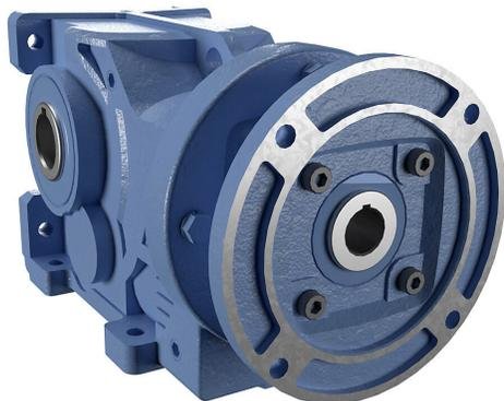
IronHorse heavy-duty helical bevel gearbox, 40:1 ratio, 143/5TC-Face input, hollow, 1.375in diameter output shaft, nominal 2hp at 1.25 SF, 3372 lb-in mechanical output torque, Type-47 frame, cast iron housing, vertical or horizontal mount.
