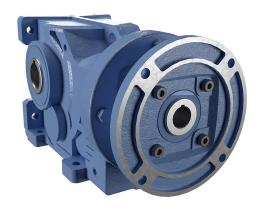
IronHorse heavy-duty helical bevel gearbox, 40:1 ratio, 143/5TC-Face input, hollow, 1.375in diameter output shaft, nominal 2hp at 1.25 SF, 3372 lb-in mechanical output torque, Type-47 frame, cast iron housing, vertical or horizontal mount.
