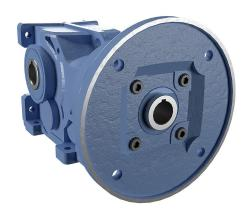
IronHorse heavy-duty helical bevel gearbox, 20:1 ratio, 182TC-Face input, hollow, 1.375in diameter output shaft, nominal 3hp at 1.32 SF, 2675 lb-in mechanical output torque, Type-47 frame, cast iron housing, vertical or horizontal mount.
