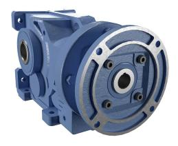
IronHorse heavy-duty helical bevel gearbox, 20:1 ratio, 143/5TC-Face input, hollow, 1.375in diameter output shaft, nominal 2hp at 1.99 SF, 2675 lb-in mechanical output torque, Type-47 frame, cast iron housing, vertical or horizontal mount.
