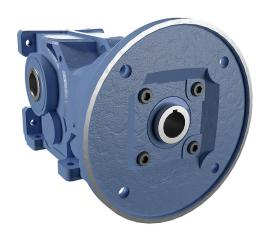
IronHorse heavy-duty helical bevel gearbox, 10:1 ratio, 182/4TC-Face input, hollow, 1.375in diameter output shaft, nominal 5hp at 1.29 SF, 2097 lb-in mechanical output torque, Type-47 frame, cast iron housing, vertical or horizontal mount.
