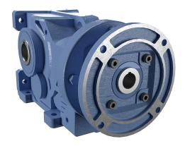
IronHorse heavy-duty helical bevel gearbox, 10:1 ratio, 143/5TC-Face input, hollow, 1.375in diameter output shaft, nominal 2hp at 3.23 SF, 2097 lb-in mechanical output torque, Type-47 frame, cast iron housing, vertical or horizontal mount.
