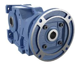
IronHorse heavy-duty helical bevel gearbox, 40:1 ratio, 143TC-Face input, hollow, 1.25in diameter output shaft, nominal 1hp at 1.43 SF, 1770 lb-in mechanical output torque, Type-37 frame, cast iron housing, vertical or horizontal mount.
