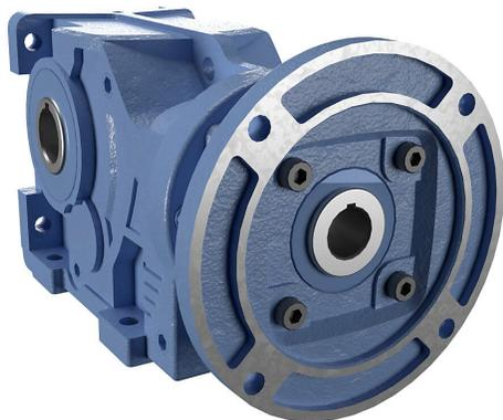
IronHorse heavy-duty helical bevel gearbox, 25:1 ratio, 143/5TC-Face input, hollow, 1.25in diameter output shaft, nominal 2hp at 1.1 SF, 1659 lb-in mechanical output torque, Type-37 frame, cast iron housing, vertical or horizontal mount.
