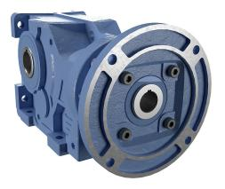
IronHorse heavy-duty helical bevel gearbox, 25:1 ratio, 143/5TC-Face input, hollow, 1.25in diameter output shaft, nominal 2hp at 1.1 SF, 1659 lb-in mechanical output torque, Type-37 frame, cast iron housing, vertical or horizontal mount.
