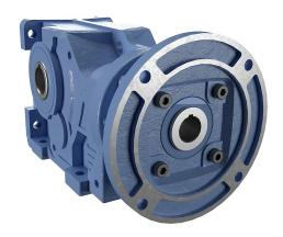
IronHorse heavy-duty helical bevel gearbox, 10:1 ratio, 143/5TC-Face input, hollow, 1.25in diameter output shaft, nominal 2hp at 2.17 SF, 1565 lb-in mechanical output torque, Type-37 frame, cast iron housing, vertical or horizontal mount.
