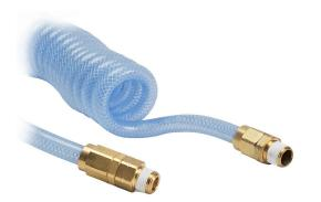
NITRA pneumatic coiled hose, polyurethane, polyester reinforced, clear blue, 3/8in inside diameter, 0.5625in outside diameter, 3/8in male NPT brass fittings (one end fixed, one end swivel), 12ft working length.
