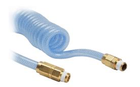
NITRA pneumatic coiled hose, polyurethane, polyester reinforced, clear blue, 3/8in inside diameter, 0.5625in outside diameter, 3/8in male NPT brass fittings (one end fixed, one end swivel), 8ft working length.
