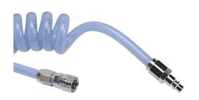
NITRA pneumatic coiled hose, polyurethane, polyester reinforced, clear blue, 3/8in inside diameter, 0.5625in outside diameter, 3/8in chrome plated steel quick-disconnect fittings, 8ft working length.
