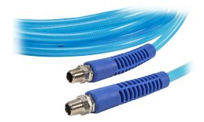
NITRA pneumatic hose, ether-based polyurethane, polyester reinforced, clear blue, 3/8in inside diameter, 0.5625in outside diameter, 1/4in male NPT nickel-plated brass swivel fittings, 50ft package.
