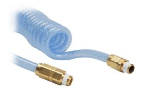
NITRA pneumatic coiled hose, polyurethane, polyester reinforced, clear blue, 1/4in inside diameter, 0.375in outside diameter, 1/4in male NPT brass fittings (one end fixed, one end swivel), 12ft working length.
