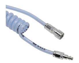
NITRA pneumatic coiled hose, polyurethane, polyester reinforced, clear blue, 1/4in inside diameter, 0.375in outside diameter, 1/4in chrome plated steel quick-disconnect fittings, 12ft working length.
