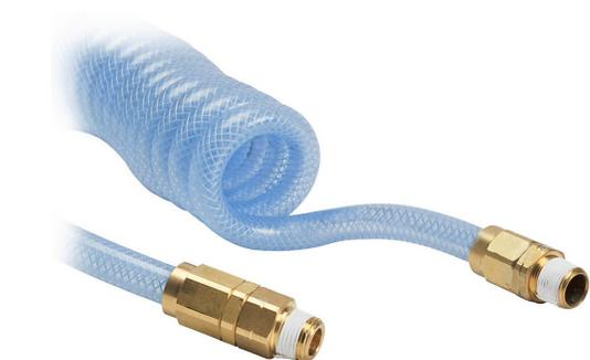
NITRA pneumatic coiled hose, polyurethane, polyester reinforced, clear blue, 1/4in inside diameter, 0.375in outside diameter, 1/4in male NPT brass fittings (one end fixed, one end swivel), 8ft working length.
