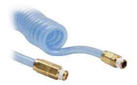
NITRA pneumatic coiled hose, polyurethane, polyester reinforced, clear blue, 1/4in inside diameter, 0.375in outside diameter, 1/4in male NPT brass fittings (one end fixed, one end swivel), 8ft working length.
