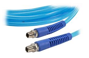
NITRA pneumatic hose, ether-based polyurethane, polyester reinforced, clear blue, 1/4in inside diameter, 0.375in outside diameter, 1/4in male NPT nickel-plated brass swivel fittings, 50ft package.
