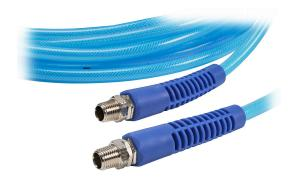
NITRA pneumatic hose, ether-based polyurethane, polyester reinforced, clear blue, 1/4in inside diameter, 0.375in outside diameter, 1/4in male NPT nickel-plated brass swivel fittings, 25ft package.
