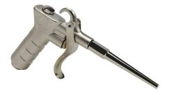
NITRA pneumatic blow gun, pistol grip, 6in nozzle, cast aluminum, 1/4in female NPT.
