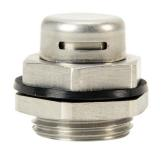
Bimed pressure relief vent plug, M20 x 1.5mm thread type, stainless steel, 2,000 mL/min @ 70 mBar (1 psi), IP67 IP68.
