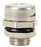
Bimed pressure relief vent plug, M12 x 1.5mm thread type, stainless steel, 2,000 mL/min @ 70 mBar (1 psi), IP67 IP68, UL Type 4X, 12 and 13.
