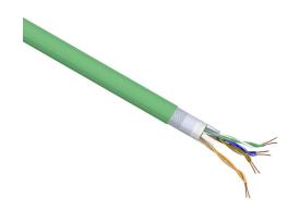
Helukabel HELUKAT continuous flexing Cat5e industrial Ethernet cable, overall shielded, 4 twisted pairs, 26 AWG, 19-stranded, bare copper, polyolefin conductor insulation material, PUR jacket, green, cut to length.
