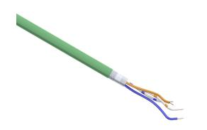
Helukabel HELUKAT continuous flexing Cat5e industrial Ethernet cable, overall shielded, 1 star quad, 26 AWG, 19-stranded, bare copper, polyolefin conductor insulation material, PUR jacket, green, cut to length.
