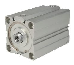
NITRA pneumatic cylinder, compact extruded, 80mm bore, 25mm rod diameter, 100mm stroke, double acting, magnetic piston, tapped end caps mount.
