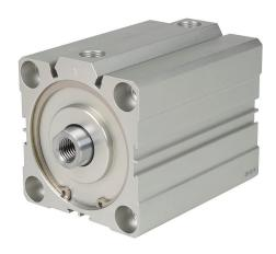
NITRA pneumatic cylinder, compact extruded, 80mm bore, 25mm rod diameter, 75mm stroke, double acting, magnetic piston, tapped end caps mount.
