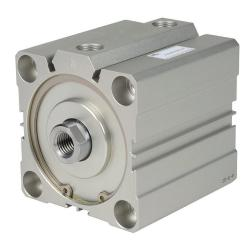
NITRA pneumatic cylinder, compact extruded, 80mm bore, 25mm rod diameter, 50mm stroke, double acting, magnetic piston, tapped end caps mount.
