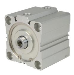
NITRA pneumatic cylinder, compact extruded, 80mm bore, 25mm rod diameter, 40mm stroke, double acting, magnetic piston, tapped end caps mount.
