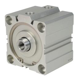
NITRA pneumatic cylinder, compact extruded, 80mm bore, 25mm rod diameter, 30mm stroke, double acting, magnetic piston, tapped end caps mount.
