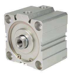
NITRA pneumatic cylinder, compact extruded, 80mm bore, 25mm rod diameter, 25mm stroke, double acting, magnetic piston, tapped end caps mount.
