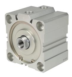
NITRA pneumatic cylinder, compact extruded, 80mm bore, 25mm rod diameter, 20mm stroke, double acting, magnetic piston, tapped end caps mount.
