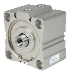
NITRA pneumatic cylinder, compact extruded, 80mm bore, 25mm rod diameter, 15mm stroke, double acting, magnetic piston, tapped end caps mount.
