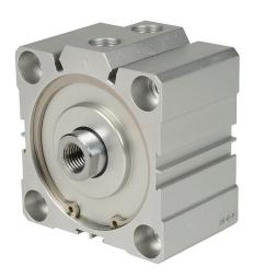
NITRA pneumatic cylinder, compact extruded, 80mm bore, 25mm rod diameter, 10mm stroke, double acting, magnetic piston, tapped end caps mount.
