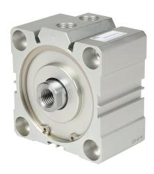
NITRA pneumatic cylinder, compact extruded, 80mm bore, 25mm rod diameter, 5mm stroke, double acting, magnetic piston, tapped end caps mount.
